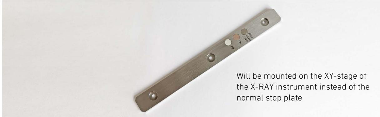
Will be mounted on the XY-stage of
